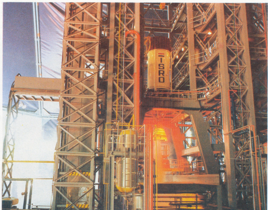
Simulation of firing of second stage liquid engine for PSLV.
