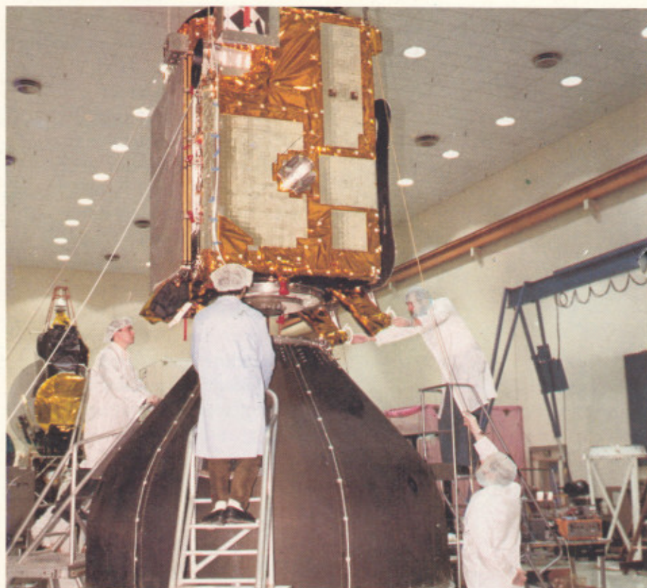
INSAT-IC being assembled on to the launch vehicle adaptor.
