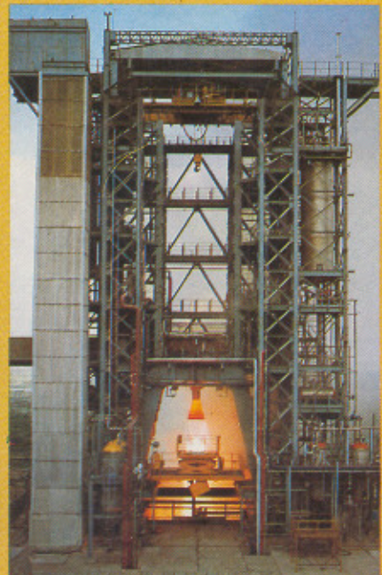
Vikas engine undergoing a long duration test.
