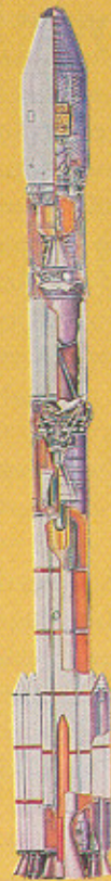
The Polar Satellite Launch Vehicle (PSLV) whose second stage will be powered by the Vikas engine.
