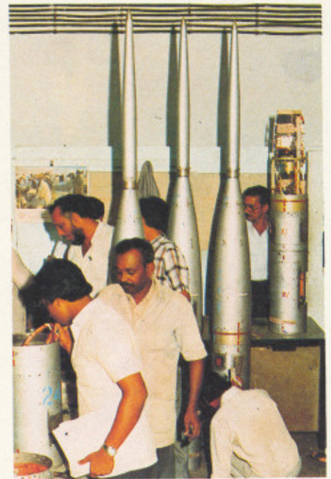
Indian Ozonesonde payloads being assembled for the 'Ozone Campaign'
