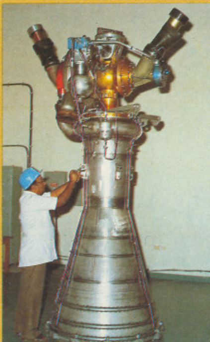
Vikas engine fully integrated and getting ready for static tests.
