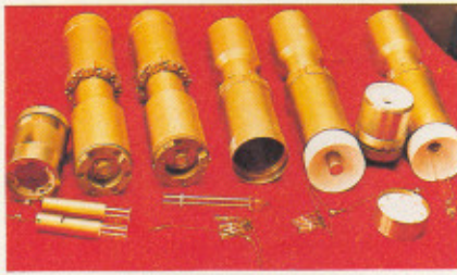
Exploded view of the Soviet gasphase chemiluminescent ozonesonde used during the intercomparison experiments.
