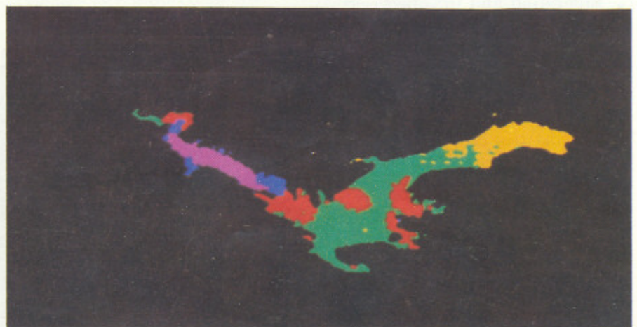
Classified image of the lake shows different levels of turbidity. (Pink, blue, red, yellow and green colours reveal high to low turbidity in that order).
