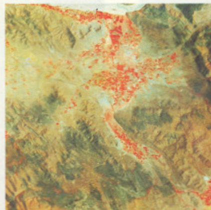
Principal component transformation of the TM bands show the lithology of the area prominently.
