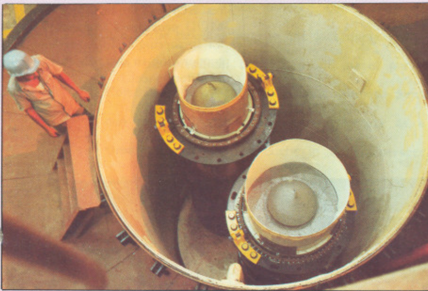
A solid rocket motor case Insulation getting ready for curing in the autoclave
