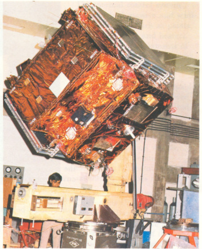
Moment of Inertia Measurements being carried out on the Engineering model of the IRS
