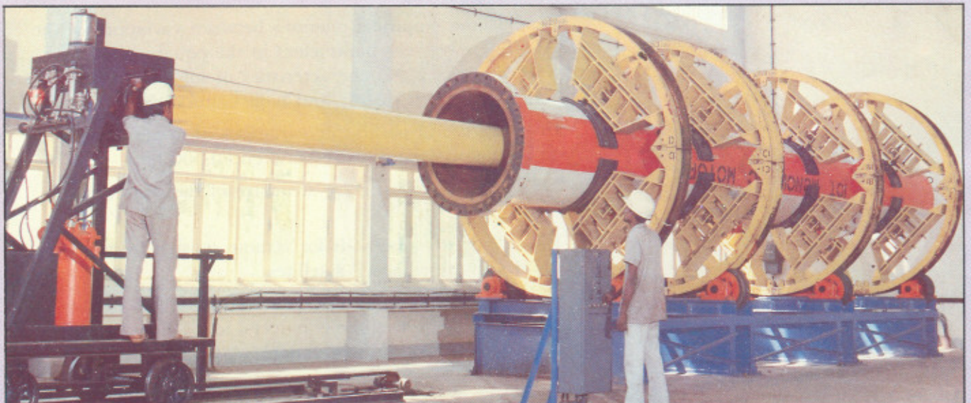
Application of resin liner to a rocket chamber
