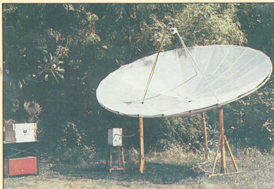
Radio networking receive terminal developed by the Space Applications Centre (SAC) for use with INSAT: The technology for the terminal has been transferred to a public sector industry for manufacture.
