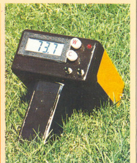
Portable Agrophotometer for the measurement of water content and chlorophyll concentration in plant leaves: The technology for this in situ measurement device developed at the ISRO Satellite Centre (ISAC) has been transferred to an industry for mass production.
