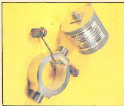
Thrust Transducer for space applications developed by the Vikram Sarabhai Space Centre (VSSC): A private sector industry has been licensed for the manufacture of the transducer.
