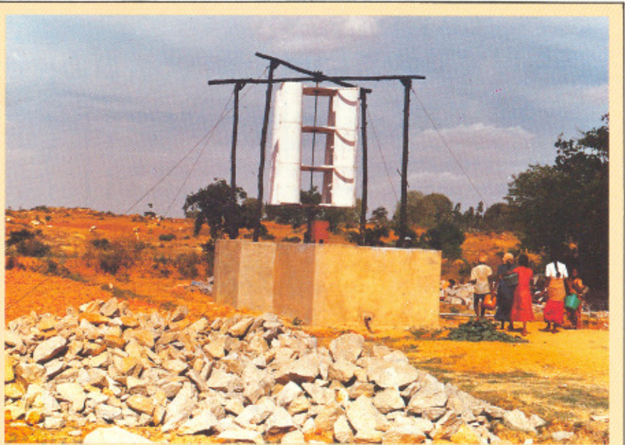
Rural Windmill for pumping water developed by the INSAT Master Control Facility (MCF), and installed at Seegenahalli Village, Mulbagal Taluk in Karnataka: This technology has since been transferred to industry.
