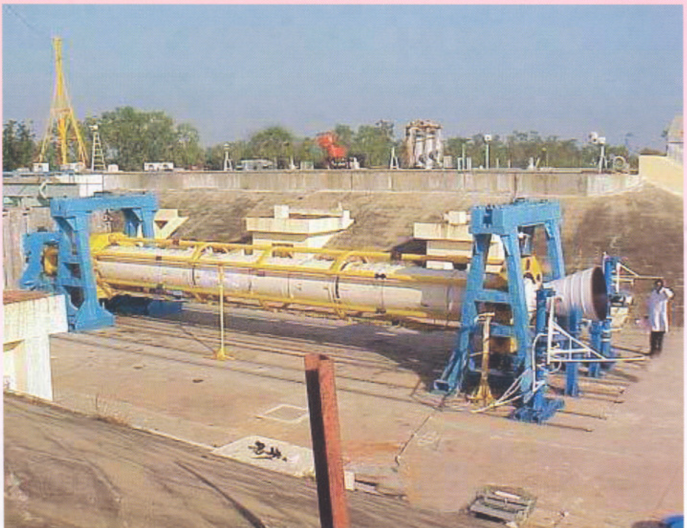
PSOM-XL in its static test stand
