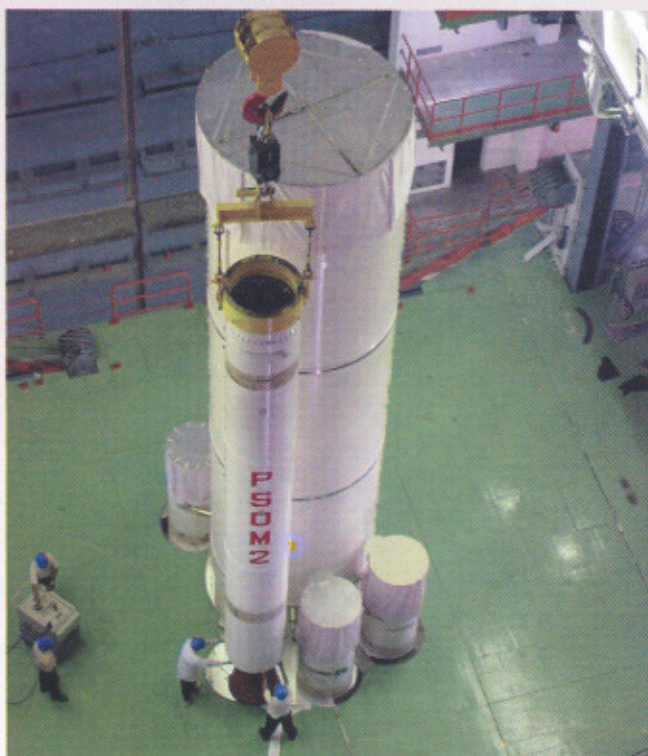
One of the strap-on motors being integrated with PSLV-C6 first stage
