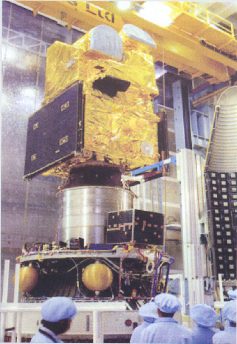
Launching two Indian Satellites at a time – the larger CARTOSAT-1 (top) with the piggyback satellite HAMSAT (in the middle) mounted on PSLV-C6 fourth stage
