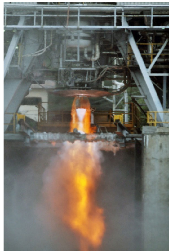
High Thrust cryogenic rocket engine undergoing heat testing
