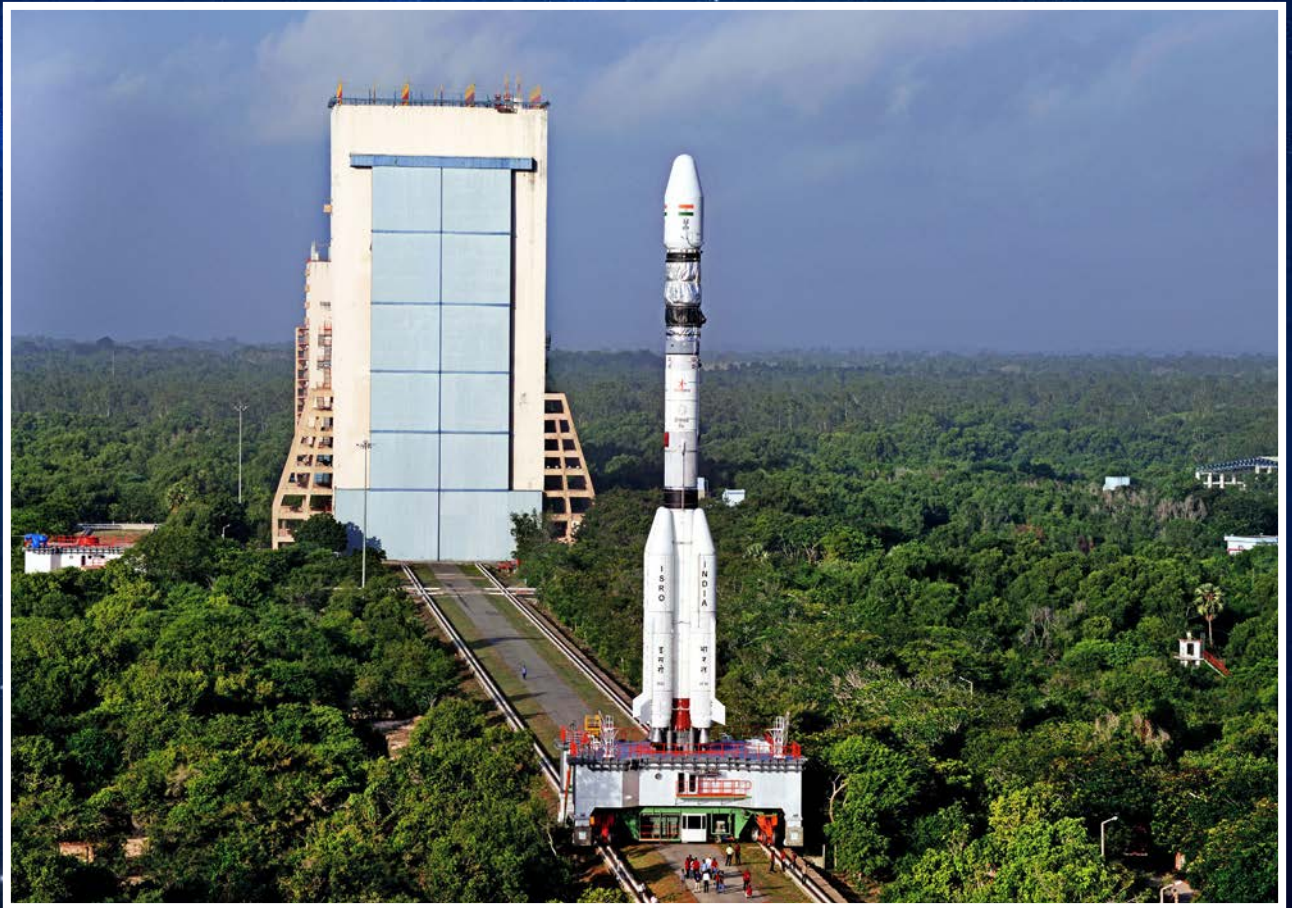
GSLV-D6 carrying GSAT-6 is being moved from Vehicle Assembly Building to Launch Pad
