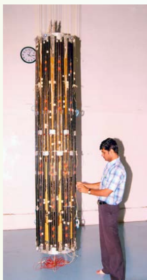
Unfurlable Antenna of GSAT-6 in stowed mode
