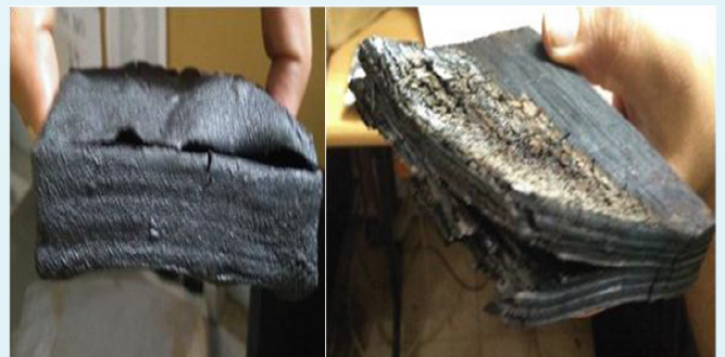
Coated v/s bare wood specimen at 400°C
