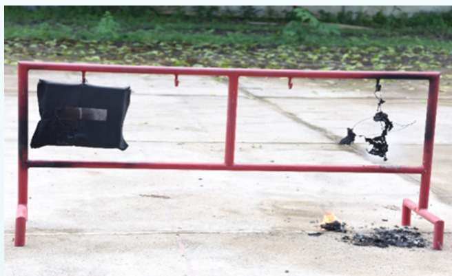
Fig. 3 Two images of commercial seat cushion set to fire. In each image: (Left)-cushion with CASPOL impregnation remain intact even after fire whereas cushion without CASPOL impregnation (Right) is burned completely in fire within a few seconds
