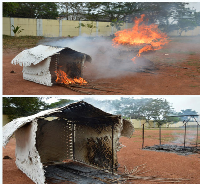
Fig. 1 Model huts made of thatched coconut leaves set to fire. (Left)-Hut without CASPOL coating gutted completely in fire within a few seconds whereas CASPOL coated hut remained intact even in fire.
