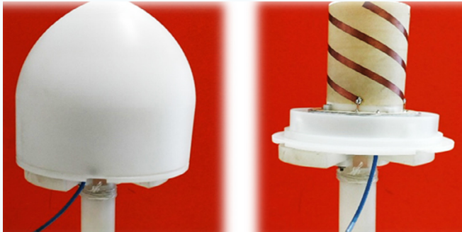
Tx Antenna for Pole
