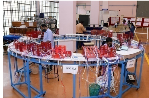
Figure 2.6: IS1/2M subassembly harness (LVM3)
