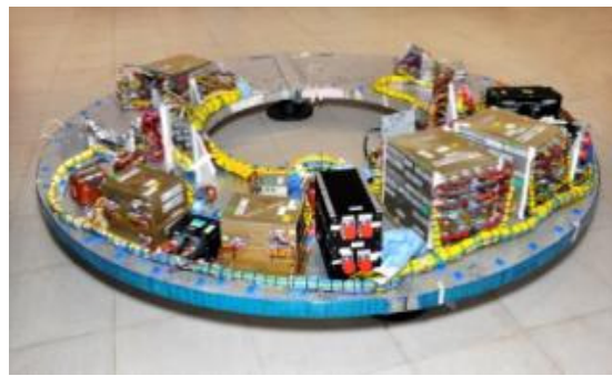
Figure 2.7: Equipment bay subassembly harness (LVM3)
