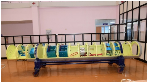
Figure 2.5: SES subassembly (LVM3)
