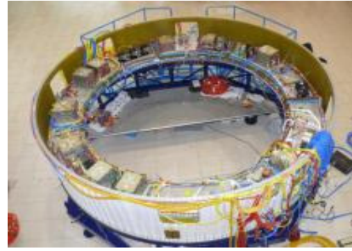
Figure 2.8: IS1/2M sub-assembly (LVM3)
