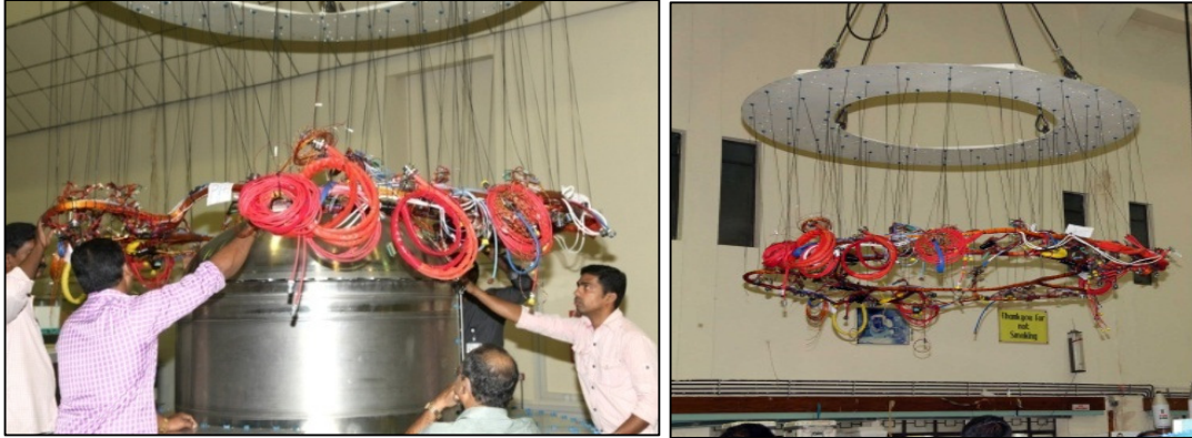
Fig. 3.5.2: Harness transfer to flight hardware
