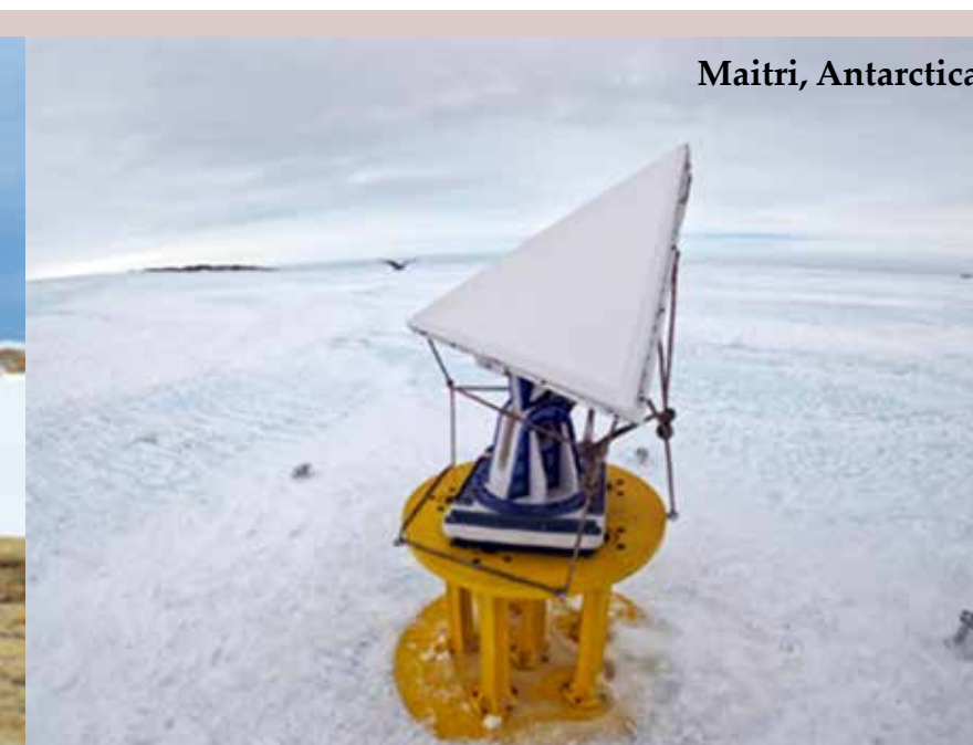
Maitri, Antarctica Corner Reflectors Installed at Antarctica (Synthetic Aperture Radar (SAR) Calibration Site)
