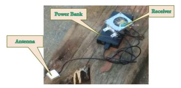
Figure-3: NavIC Messaging and Positioning Receiver Setup with power bank and Antenna
