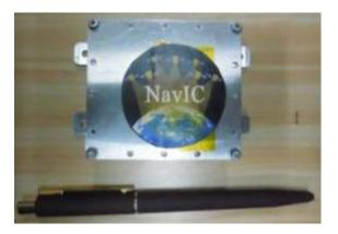
Figure-2: NavIC Messaging and Positioning Receiver
