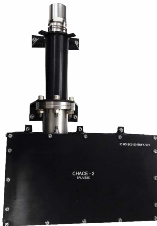
Figure 2.10: FM of the CHACE-2 instrument
